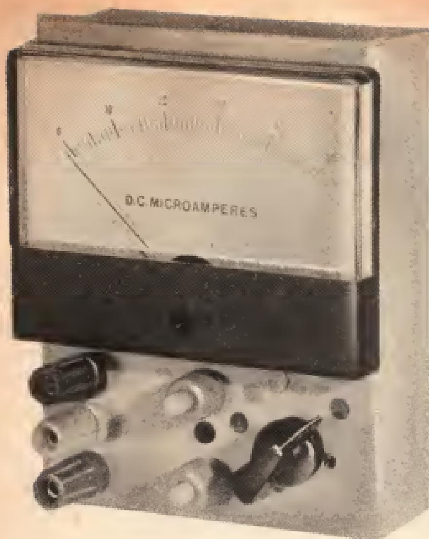
from base to collector, but not in reverse or from collector to emitter. A *pnp* transistor will conduct only from emitter or collector to base. When connected for conduction, the meter will indicate some resistance less than f.s.d. When otherwise connected, a greater resistance (usually greater than f.s.d.) will be shown.
